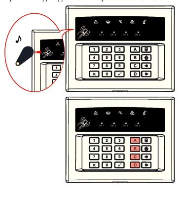
the 1-4 numeric keys have been pressed. Once illuminated, it signifies that the output has triggered. Press the key again to deactivate the output.
