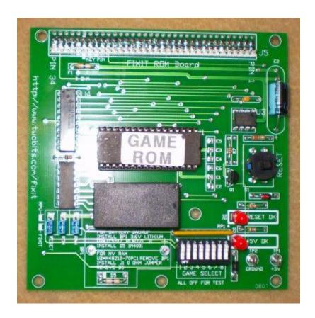
The FIXIT board contains the software for all Bally and Stern pinball machines manufactured from 1977 through 1985. Game selection is made by setting the DIP
