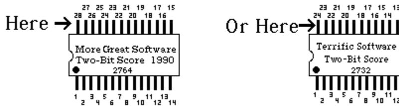
The Negative (Ground) is delivered to the pin in the OPPOSITE corner!
