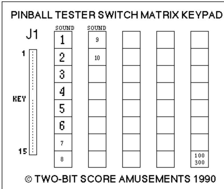
If you are working on an SB-300 Sound board, press the 100-300 button to enter the SB-300 test mode.
