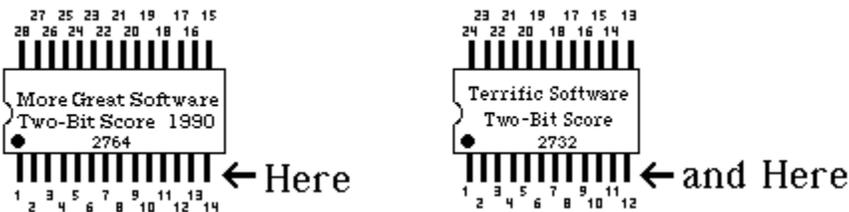
If you do not observe the polarity when you plug in the chips, you will deliver negative voltage directly to the positive pin, and positive voltage to the negative pin.
