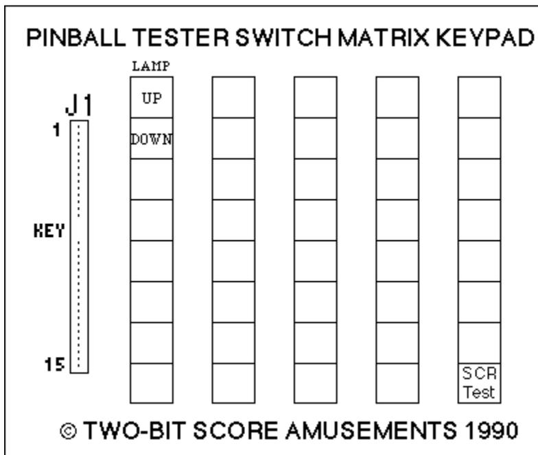
If a large number of lamps are not functioning, and you have confirmed that the bulbs are good and receiving power, look for signal being generated at PIA U10 pins 2 - 9 and continuity to J1 pins 12 - 19.
