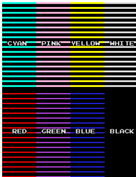
The Color Bar Test with PACPLUS Color PROMs Note that the GREEN bar appears PURPLE.
