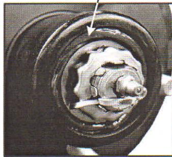
Hub cavity is full when the HYBRID-OIL lubricant first appears around edge of spindle washer. Remove grease fitting.
