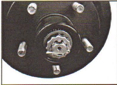
Install hub nose O-ring & adjust bearings per UFP Assembly Instructions.\*
