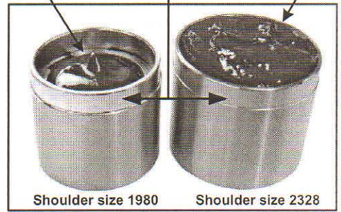
Fill THE VAULT protector cap with HYBRID-OIL lubricant. As shown in the photo above. Apply "Loctite" retaining compound to shoulder of protector.
