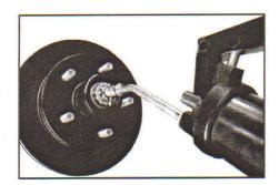
Fill hub cavity with the HYBRID-OIL lubricant. Rotate hub during filling to disperse air.
