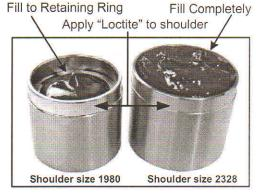
Fill THE VAULT protector cap with HYBRID-OIL lubricant. As shown in the photo above. Apply "Loctite" retaining compound to shoulder of protector.
