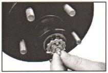
Screw a 1/8" NPT (Auto parts store) grease fitting into the threaded hole in the end of the spindle.
