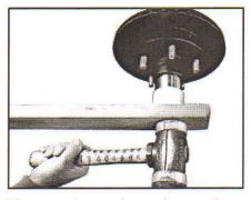
Place a piece of wood over the collar and hit with a mallet to drive the protector STRAIGHT into the hub. You can expect excess HYBRID-OIL to escape from the sides of the protector.
