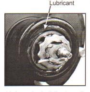
Hub cavity is full when the HYBRID-OIL lubricant first appears around edge of spindle washer. Remove grease fitting.
