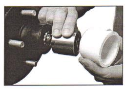
Place PVC collar over protector (2"x1-½" slip collar for 1980 size) (2" female adapter for 2328 size) in order to prevent damage to the protector during installation.
