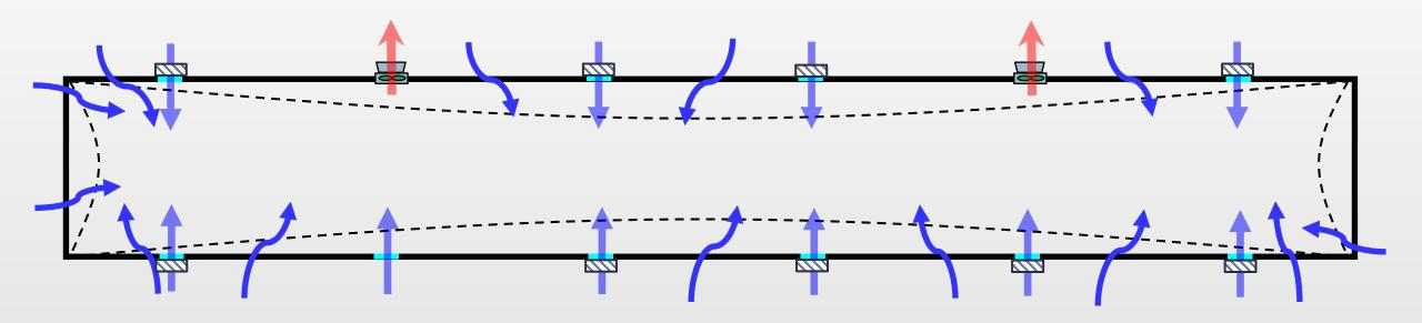
▶ 12,500 cmh of 25,000 (50%) will enter unfiltered through cracks
