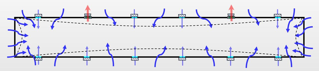
▶ 20,000 cmh+ (80%+) will enter through the cracks, unfiltered
