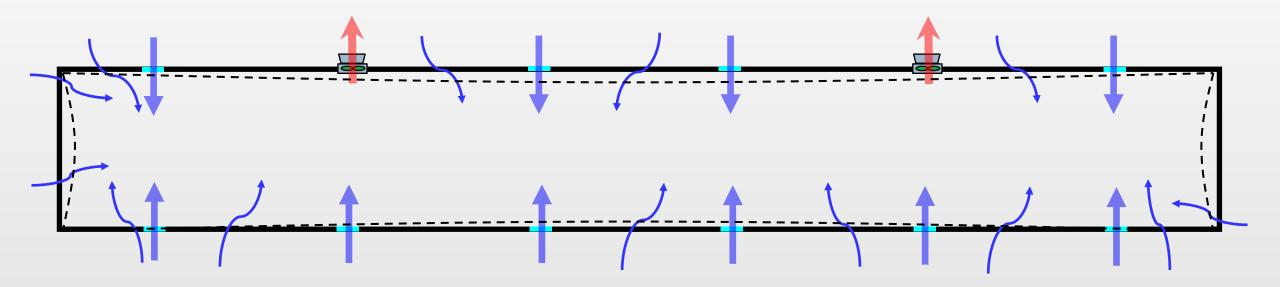
> 9,500 cmh of 25,000 (34%) will enter the house through cracks during minimum ventilation
