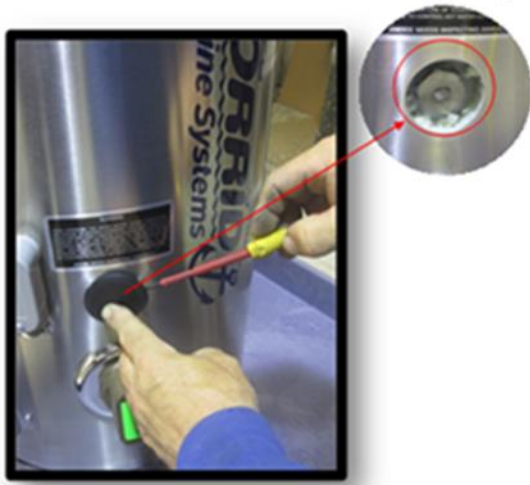
Image 1.1 Locate anode and remove plastic cover.
