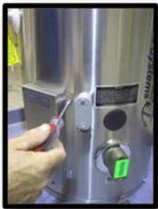
Fig. 2.1 Remove the electrical access panel door.
