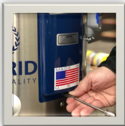
Fig. 2.1 Remove the electrical access panel door.
