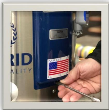
**Fig. 2.1** Remove the electrical access panel door.
