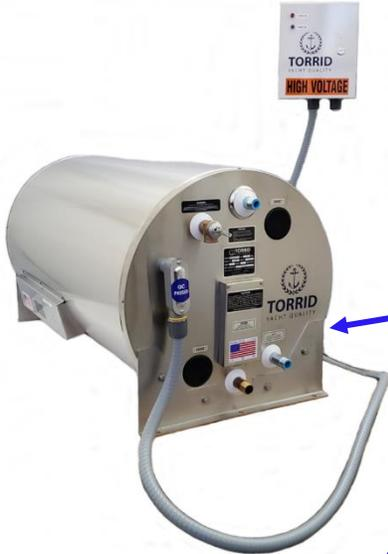
**3-Phase Water Heaters** Horizontal and Vertical 30, 40, 50, 65 & 80 gallon configurations are available. These have three heating elements and external electrical control boxes with fused breakers. A 10 ft cord connects the water heater to the control box. Each build is considered a custom build to match the 3-Phase Power of the vessel. Heat Exchangers are possible on most models as well.
