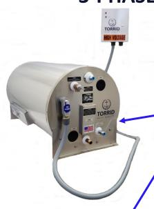
**3-Phase Water Heaters** Horizontal and Vertical 30, 40, 50, 65 & 80 gallon configurations are available. These have three heating elements and external electrical control boxes with fused breakers. A 10 ft cord connects the water heater to the control box. Each build is considered a custom build to match the 3-Phase Power of the vessel. Heat Exchangers are possible on most models as well.
