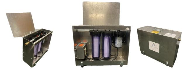
The NEW Aerospace America Compact Water Filtration Pump is light, small and easily carried on the job site. This unit is 22lbs and only 7.5"x20"x15" in size. The motor is strong and efficient at 6 GPM, 60 PSI and only draws 2.1 amps at 110V. Garden hose attachments are located on the outside of the housing for easy access. Our pumps have isolation feet for quiet operation and are of the highest quality and strongest construction on the market.
