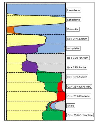
The capture spectroscopy log above shows the count rate yield for the main capture elements. The elements H, Cl and Na, which vary with porosity and salinity, are not included in the yields determination. Iron
