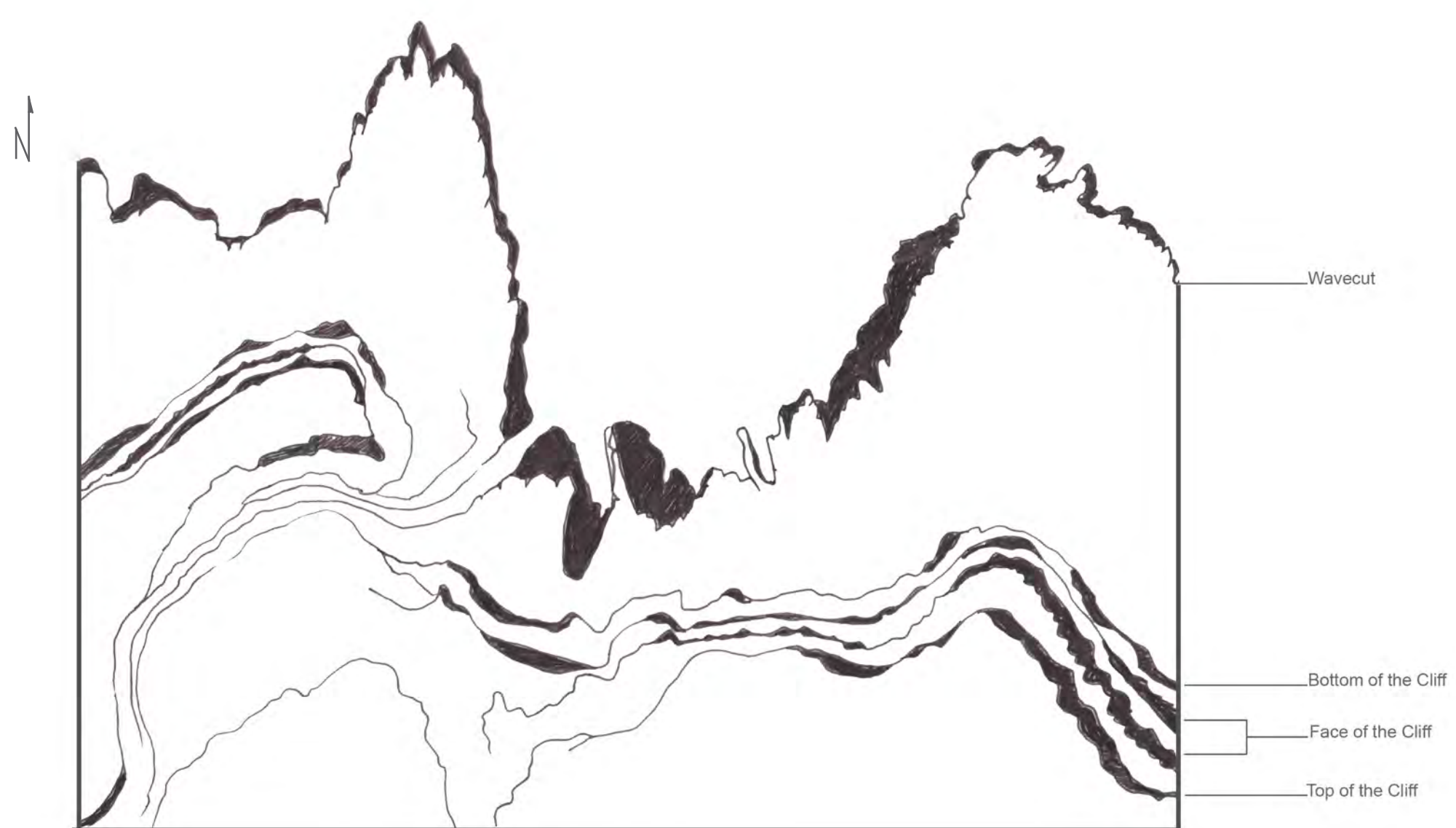
A map of Staithes tracing the movement of the Wave Cut front and the cliff through 100 years, based on historic data. Scale 1:4000
