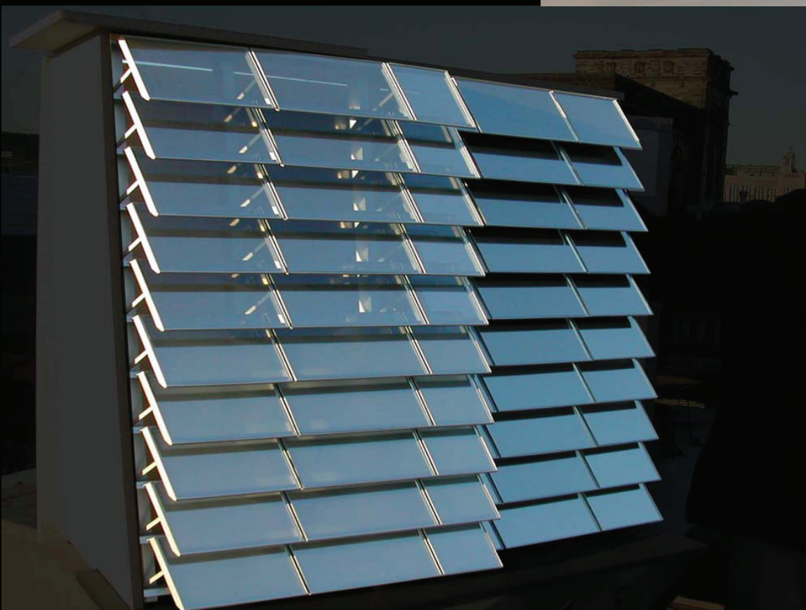
Goldman Sachs Tower- louver test Jersey City, NJ, USA Cesar Pelli and Associates 3"=1ft Scale Laser cut acrylics, SLA frames, custom painting.
