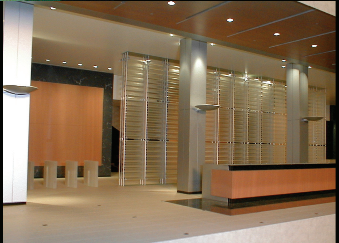
Goldman Sachs Tower- louver test Jersey City, NJ, USA Cesar Pelli and Associates 3"=1ft Scale Laser cut acrylics, SLA frames, custom painting.
