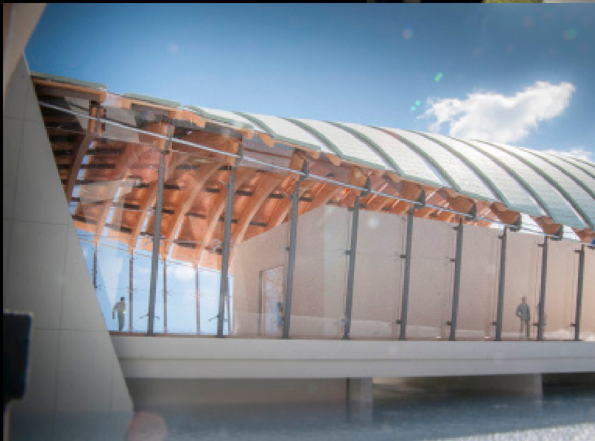
Final exhibition model Crystal Bridges Museum of American Art Bentonville, Arkansas, USA 1/4" = 1' scale Laser cut styrene and PETG, vac formed roof shell with painted styrene layers and beams. Rippled backpainted acrylic base.
