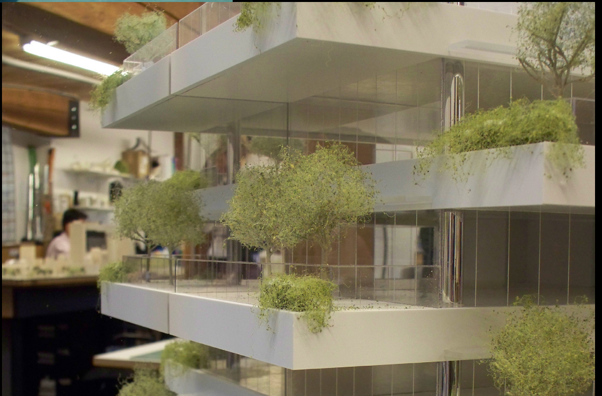
Final exhibition model Crystal Bridges Museum of American Art Bentonville, Arkansas, USA 1/4" = 1' scale Laser cut styrene and PETG, vac formed roof shell with painted styrene layers and beams. Rippled backpainted acrylic base.
