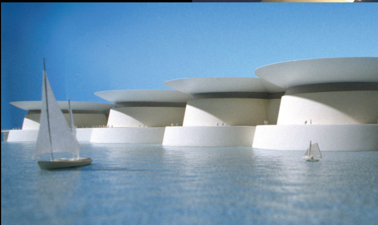
Competition model Guangdong Science Center China 1-100 scale Rippled acrylic water, styrene walkways, buildings made from vac-formed styrene, renshape and acrylic.
