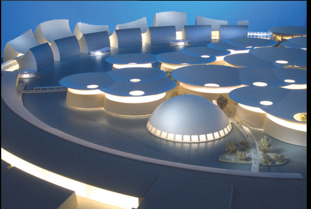
Competition model Guangdong Science Center China 1-100 scale Rippled acrylic water, styrene walkways, buildings made from vac-formed styrene, renshape and acrylic. Lighting achieved with rope light under model.
