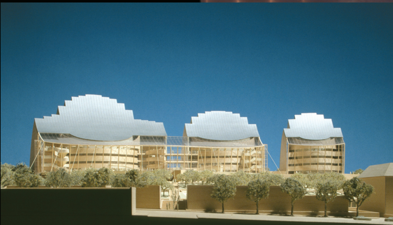
Final presentation model Kauffman Center for the Performing Arts Kansas City, MO, USA 1' = 1/8th" scale Styrene, white foam and strathmore base. Buildings are lasercut styrene and PETG. Custom hand made trees.
