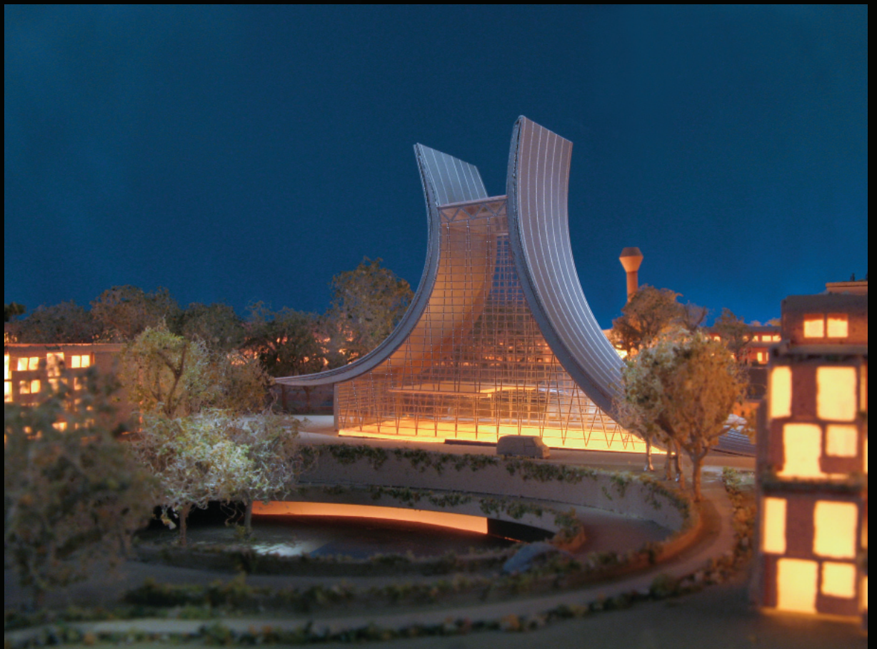
Final presentation model Danube Integrated Resort 1-500 scale Laser cut styrene and PETG, acrylic, basswood, wood veneers, custom made trees. Lighting with rope light in base. Highlights with flashlight.
