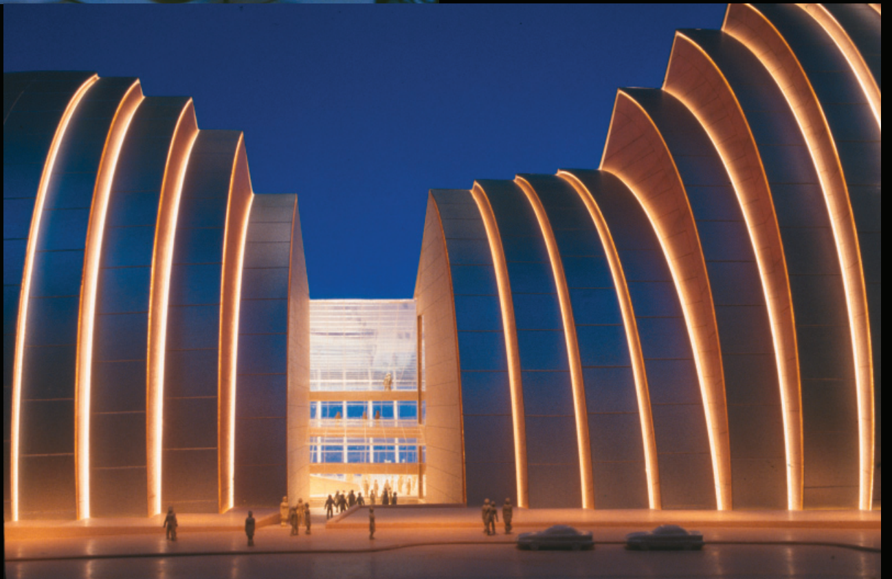
Final presentation model Kauffman Center for the Performing Arts Kansas City, MO, USA 1' = 1/8th" scale Styrene, white foam and strathmore base. Buildings are lasercut styrene and PETG. Custom hand made trees.
