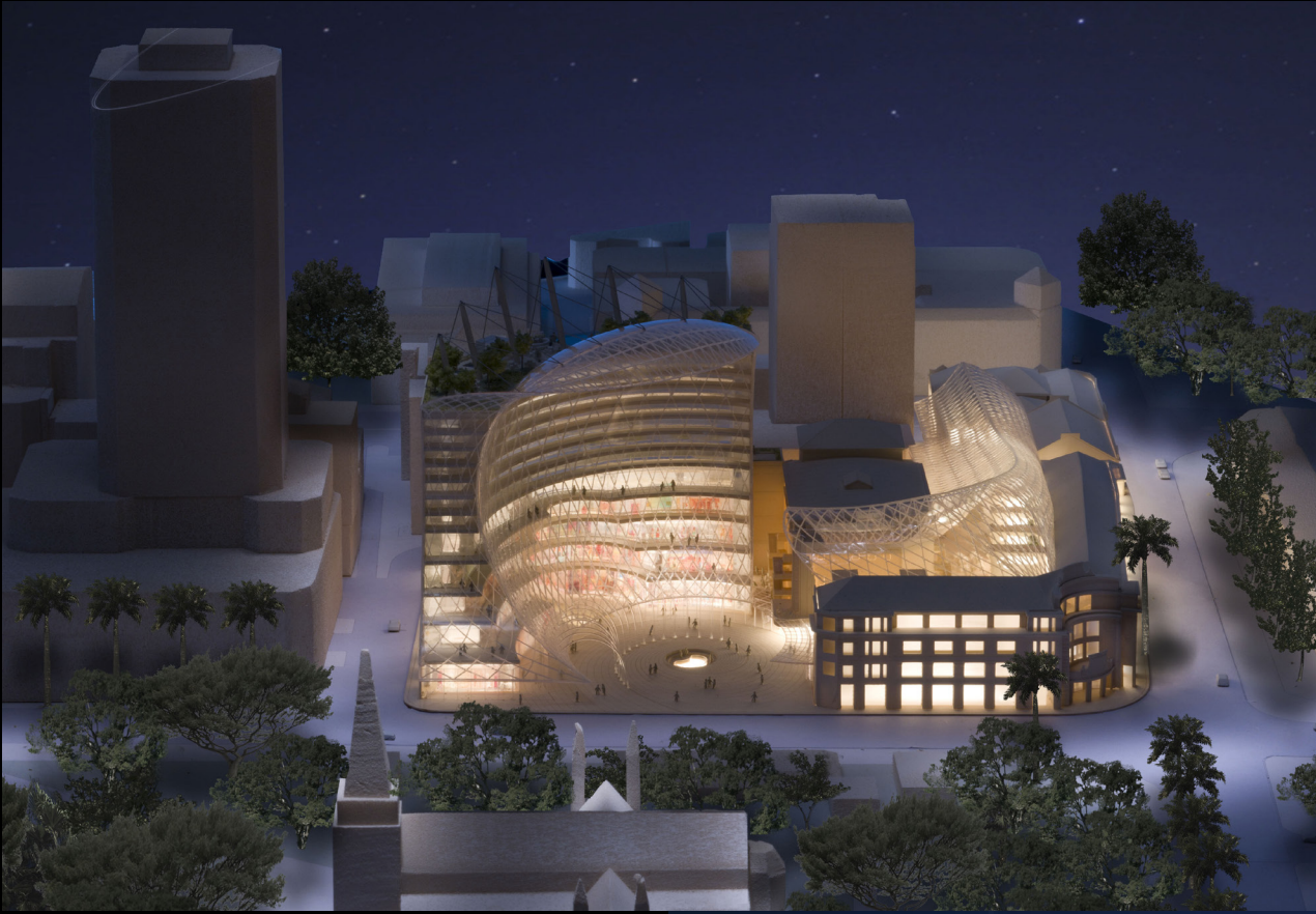
Competition model Capital Theater Singapore 1-200 scale Foam, acrylic and PETG base, solid massing buildings - basswood, main building- painted and clear lasercut PETG.
