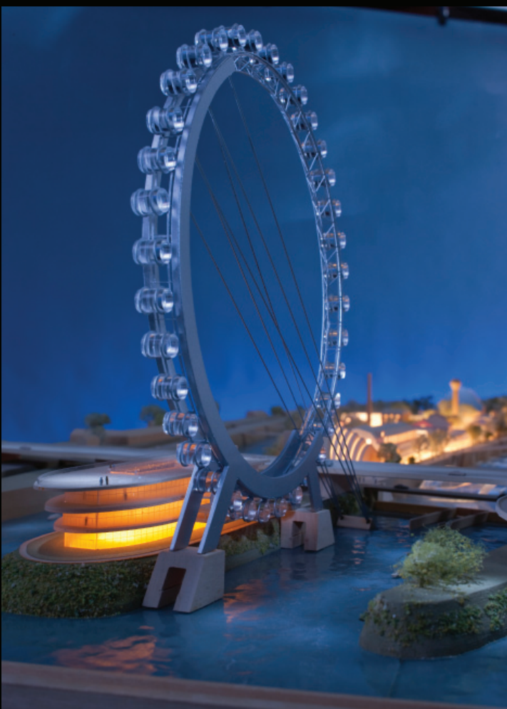
Final presentation model Danube Integrated Resort 1-500 scale Laser cut styrene and PETG, acrylic, basswood, wood veneers, custom made trees. Lighting with rope light in base. Highlights with flashlight.
