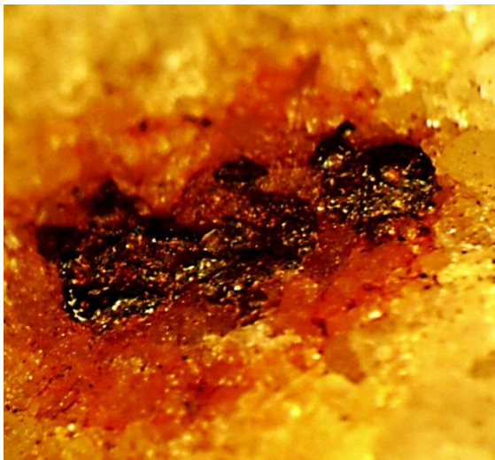
Figure 5. Iron splatter on a quartzite cobble (upper). Closer view (lower, 5 mm across).
