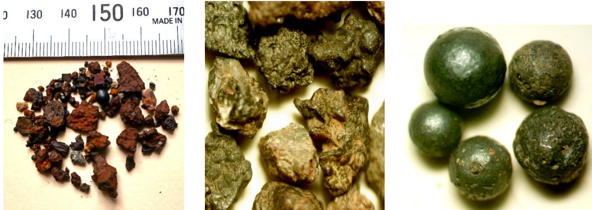
Figure 7. Hammer-scales, flaky (middle, 5 mm across) and spherical (right, 5 mm across).
