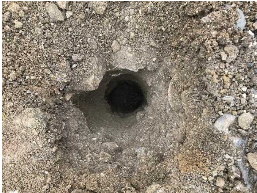
Plate 12: Bore within stockpile, showing extent of basalt cobbles, at STP09.
