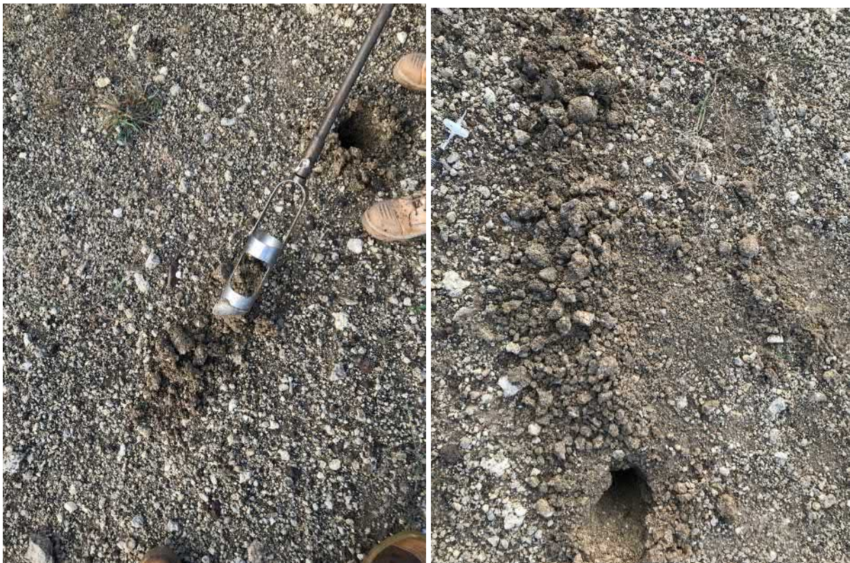
Plate 8: Sampling deep fill material at STP03.
