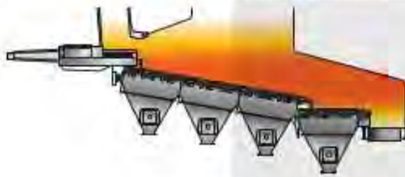
If calorific values are low, ranging from 4.5 to 11 MJ/kg, a further drop-off between zones 1 and 2 promotes drying and timely ignition.
