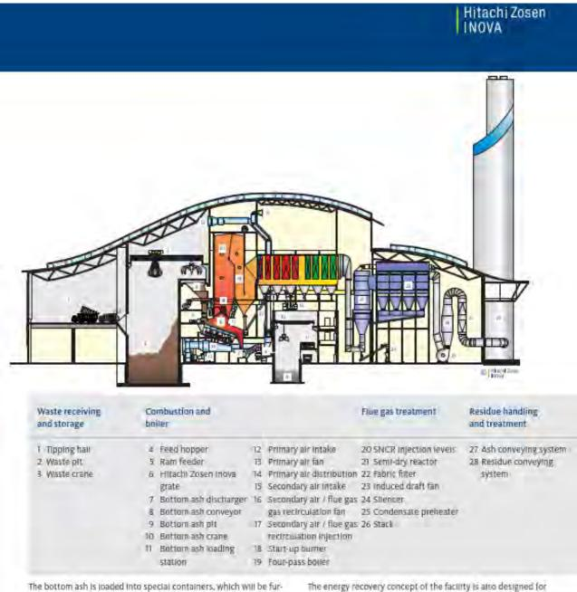
The bottom ash is loaded into special containers, which will be further transported by barges, using the same system of water transport as the waste when being delivered to the facility. All these processes take place within enclosed areas. The bottom ash is sent for processing and reuse within the construction industry, for cover material or for disposal. By means of a metal separation process, ferrous and nonferrous material is also gained for recycling purposes.
