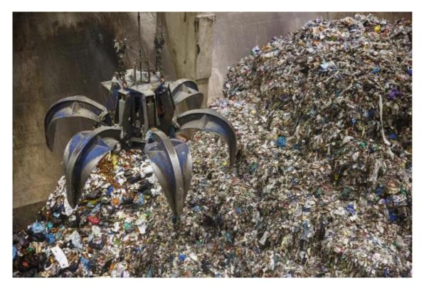
Figure 7.6: Inside a waste bunker at an EfW plant with waste feeding and mixing crane in operation
