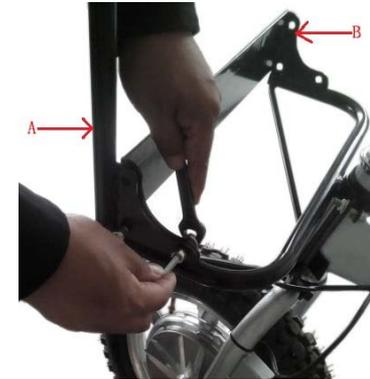
4. Install the rear frame onto the scooter with the two bolts, and tighten them with the nuts provided.
