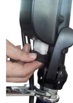
**NOTE:** Handle bar height adjustment. Handle bar height can be easily adjusted by opening the quick release on the handlebar tube to preferred height, then firmly closing quick release.
