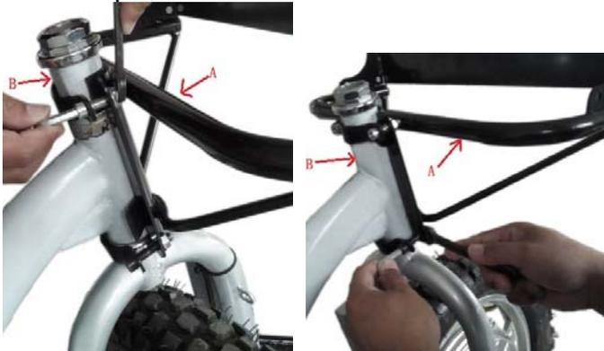
3. Put the left front frame(A) onto the front support(B), aligning the three holes, place the three bolts through the holes, then twist the bolts, and tighten them with the nuts provided. The right front frame is the same as the left front frame.
