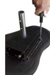
4. Install special tube on scooter, put one side with hole forward, and fasten bolts
