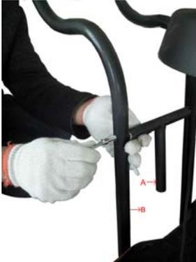
6. Fix the rear support and seat post with one bolt, and tighten them with the nuts provided.
