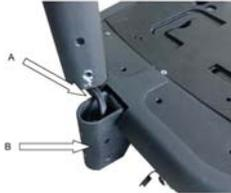
3. Remove the bolts and nuts from the connecting tube clamp (B). Place the connecting tube into the top opening (A). After aligning the holes, place the two bolts through the connecting tube and neck assembly. Twist the bolts, do not hammer them through. Tighten these two bolts with the nuts provided.
