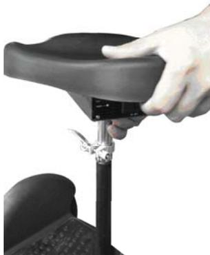
7. Put out the connecting wire harness of inverter, connect well the inverter and charger port, then tie to the post by bind.
