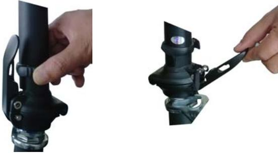
6. Ensure that the handlebar is facing front, the brake on the left side and the throttle on the right, then tighten the handlebar tube collar clamp using the enclosed 5mm wrench.
