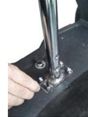
7. Align nipples to corresponding holes in floor deck
