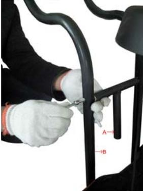
8. Fix the rear support and seat post with one bolt, and tighten them with the nuts provided.
