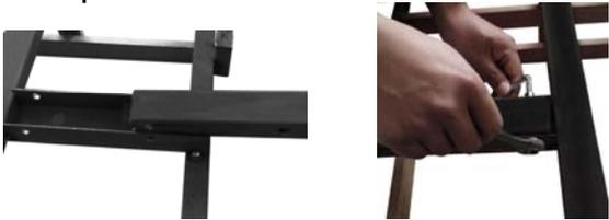
3. Place the trailer connection plate (A) into the trailer connection frame (B) of front of trailer tongue. After aligning the holes, place the trailer pin through the hole. Secure the trailer pin with the cotter pin.
