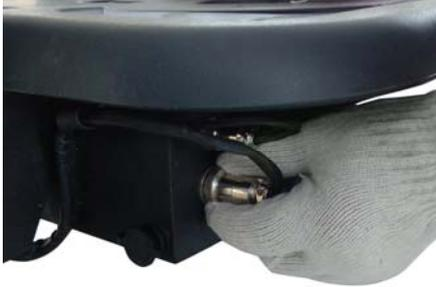
8. Match the pins of the plugs to the holes of the sockets. Note the alignment notches.
