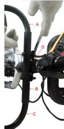
3. Fix the under-clip ring (A) onto the scooter, and tighten them with the nuts provided.
