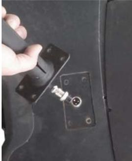
6. Install tube on scooter, put one side with hole forward, and fasten bolts
