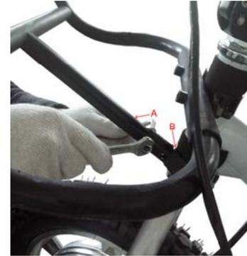
6. Install the rear frame onto the scooter with the two bolts, and tighten them with the nuts provided.
