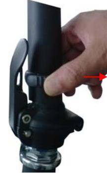
3. Press the quick release to bottom.
