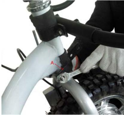
4. Install front support (A) onto front frame(B) with the two bolts, and tighten them with the nuts provided.
