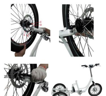
8. Install the chain. It is recommended to wear gloves for protection. Properly align chain on derailer (A). Then straighten the chain along the "B" direction and put on the crank sprocket(C). Turn the crank to verify
