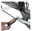
10. Insert rear brake cable through brake cable tube fixed seat(A). Then insert rear brake cable through brake cable fixed seat(B). Pull the brake cable back hard with your hand, then tighen the bolt with the provided nuts. Drive the Libert-e, slowly and test brake function.
