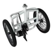
6. Remove the bolts and nuts from the connecting tube (B). Place the connecting tube into the top opening (A). After aligning the three holes, place the three bolts through the connecting tube. Twist the bolts, do not hammer them through as this can damage the threads. Tighten these three bolts with the nuts provided.
