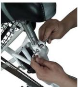
Tilt seat forward. Insert the battery and lock it. Plug the battery connector into the battery pack.
