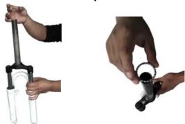
3. Put the riser of front fork into the front tube of frame, then put another ball rack into the riser of front fork. Twist the bolts and tighten it.
