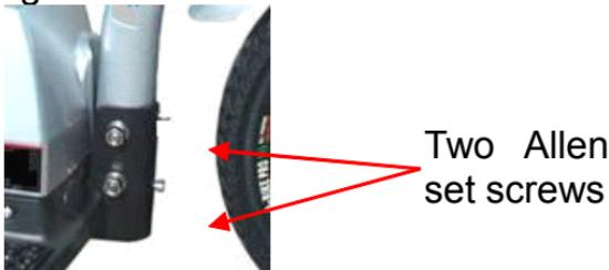
5. Extend the handle bar tube to full upright position, and slide it into connecting with the front fork.
