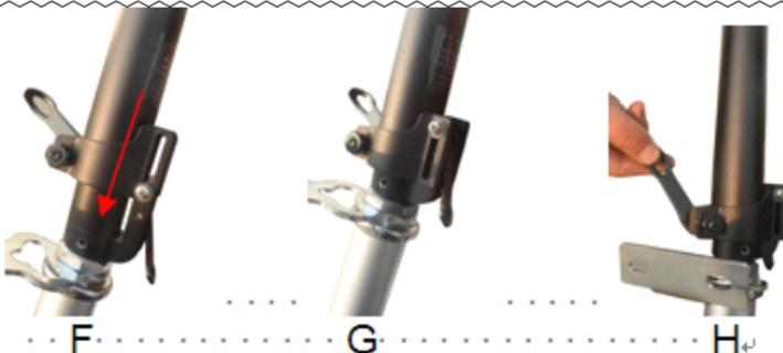
6. Ensure that the handlebar is facing front, the brake on the left side and the throttle on the right, then tighten the handlebar tube collar clamp using the enclosed 5mm wrench.
