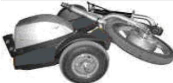
2. Place the Flex 500 on a flat, level surface. Block the front up 3.5". This will make the next step easier
