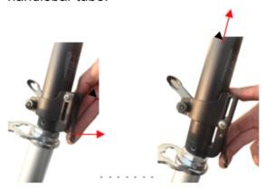
4. Lift the connecting tube (which is also attached to the handlebar tube).
