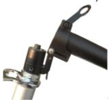
5. Carefully place the handlebar tube on the footrest frame
