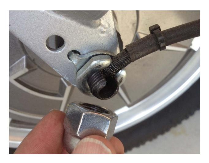
NOTE THE SLOT IN THE AXEL AND THE WASHERS ALIGNMENT FOR WIRE TO BE SECURED AT A 90 DEGREE ANGLE. TO THE MOTOR.
