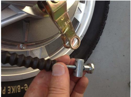
PULL CABLE TROUGH MOUNTING HOLE.
