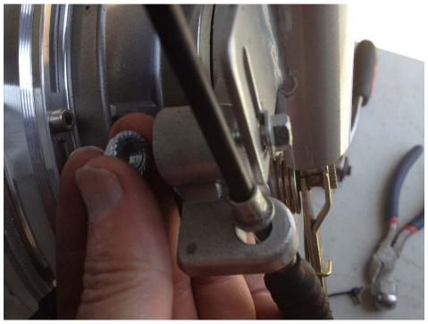
REMOVE NUT AND BOLT FROM BRAKE MOUNTING BRACKET FLANGE.
