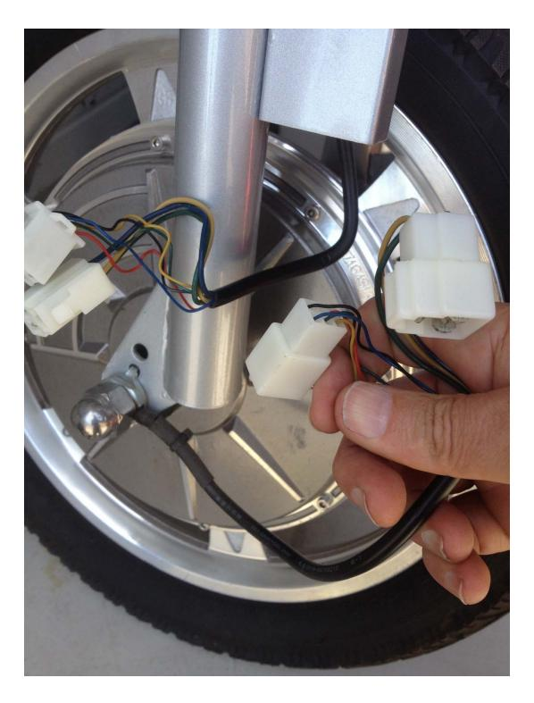
UNPLUG THE CONNECTORS. NOW THE WHEEL IS FREE FROM WIRING.
