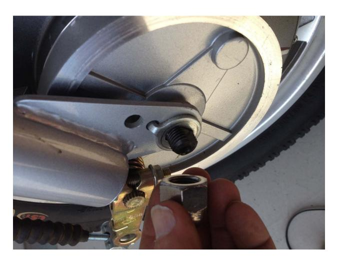
REMOVE ACORN NUT AND LOCK WASHER FROM AXEL.
