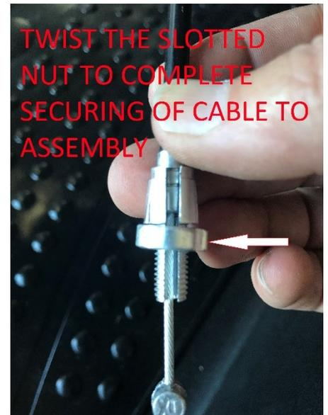
\*THE ABOVE PHOTOS ILLUSTRATE HOW THE CABLE FITS IN. ONCE THE SLOTTED NUT IS TURNED, THE CABLE CANNOT COME LOOSE.
