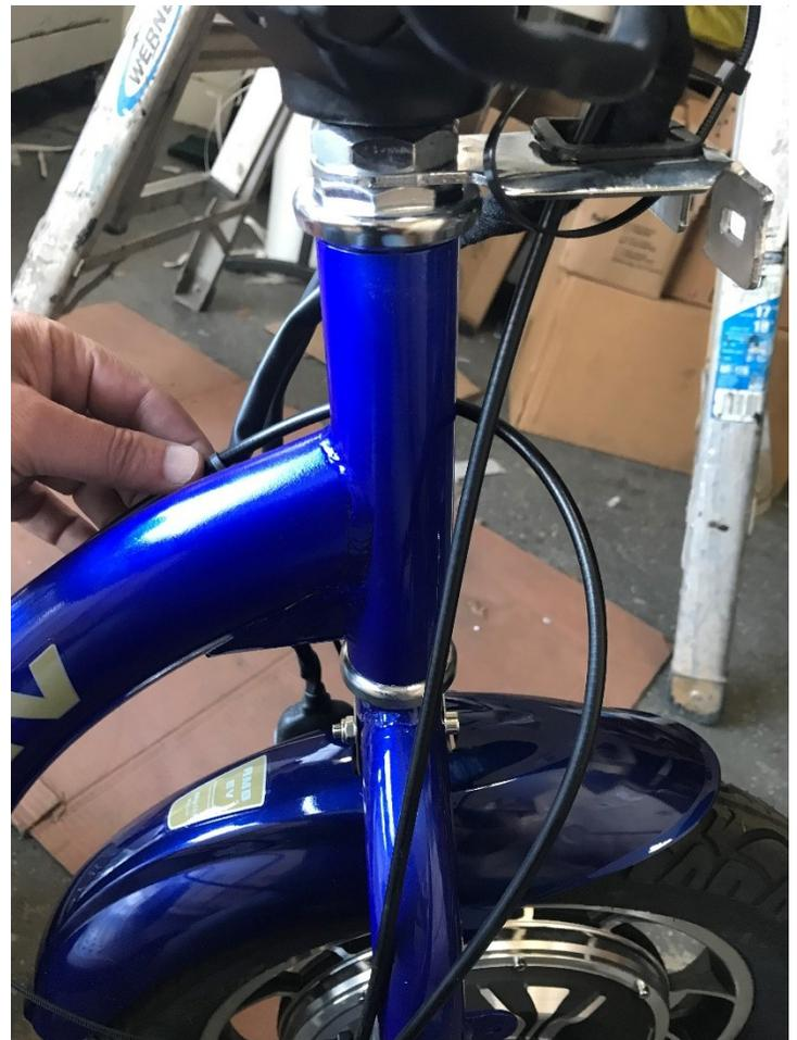
12. LOCATE THE CABLE ANCHOR ON THE FOOT BRAKE ASSEMBLY AND INSERT THE BRAKE CABLE INTO THE SLOT NOTING THAT THERE IS AN ADJUSTING NUT WITH A NOTCH IN IT THAT MUST ALIGN IN THE OPEN POSITION TO ALLOW THE CABLE TO BE INSERTED. YOU MAY NEED TO PULL THE CABLE OUT TO HAVE ENOUGH LENGTH TO SLIDE INTO PLACE.
