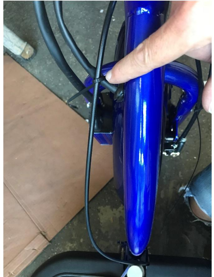
14. FOLLOW THE CABLE BACK AND TUCK THE CABLE UNDER THE PLASTIC FLOOR DECK RIM LEAVING ENOUGH SLACK FOR THE STEERING TO TURN LEFT AND RIGHT WITHOUT BINDING OR TIGHTENING TOO MUCH. WHEN FINISHED, CUT OFF EXCESS ZIP TIE.
