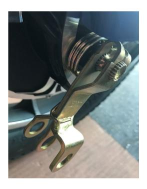
6. REMOVE THE OLD FORK BOLT TAKING NOTE THAT THERE IS A NUT THAT FITS IN A RECESS IN THE FORK FRAME THAT ALLOWS LOOSENING AND TIGHTENING WITHOUT A WRENCH ON THE BACK END.
