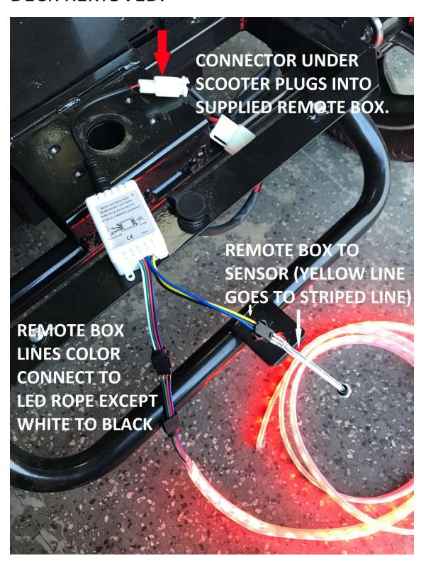
STEP 9. PAYING ATTENTION TO THE WIRING UNDER THE FLOOR DECK, ZIP TIE THE LED ROPE TO THE FRAME WITH THE LIGHTS FACING THE GROUND. THE LED ROPE WILL ATTACH TO THE BOTTOM OF THE REAR AXLE AND WRAP AROUND THE FRAME OF THE BATTERY PACK. THERE WILL BE EXCESS LED ROPE SO YOU WILL FOLD BACK UPON ITSELF AND SECURE WITH ZIP TIES. THE WHITE REMOTE BOX WILL INSTALL IN THE SEAT POST HOUSING AND SECURED BY ZIP TYING THE WIRES THAT COME OUT OF IT TO THE FRAME.
