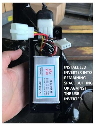
STEP 6. INSTALL THE PROVIDED LED INVERTER BEHIND THE USB INVERTER.
