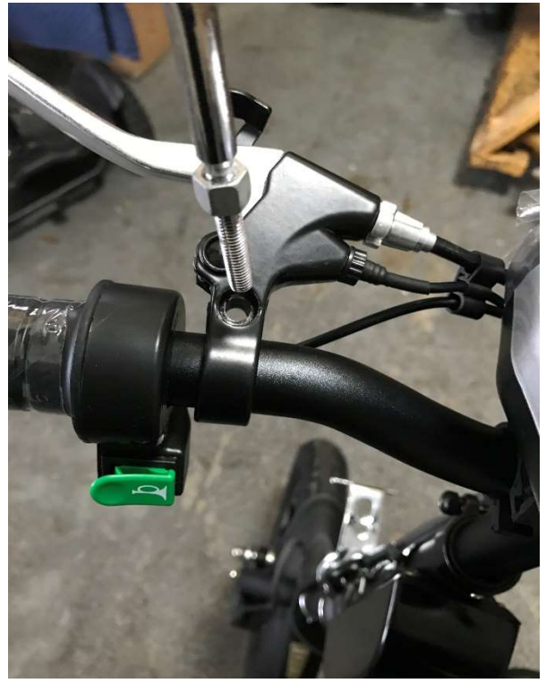
insert mirror into brake lever.
