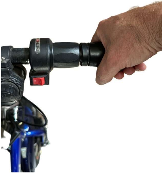
Twist the end grip while pulling
