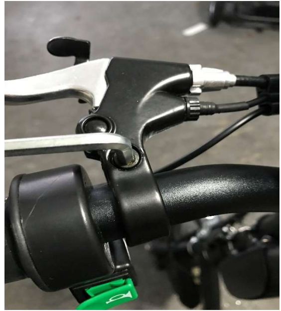
Remove allen bolt with allen Wrench.
