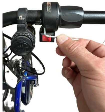
Loosen set screw and slide throttle off (you may need to loosen headlight to get off bar)
