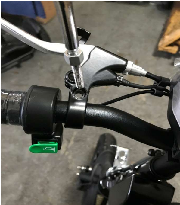
Mount to brake lever
