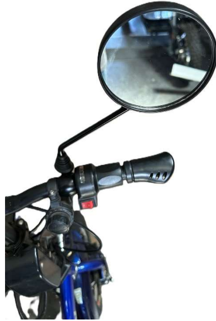
Mirror mounted with throttle and end grip reinstalled. (Be sure end grip does not physically touch throttle as this could cause throttle to get stuck)
