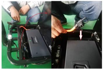
Unplug the power line from the battery pack as shown.
