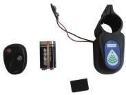
2. Connect the battery and install on seat post.
