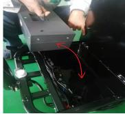
Lift battery pack using the provided handle
