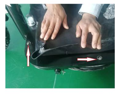
Gently peel back the edges of the rubber floor mat to access the four screws that secure the battery access panel. Unscrew the four screw and lift the access panel up.
