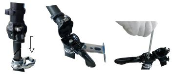
6. Ensure that the handlebar is facing front, the brake on the left and the throttle on the right, tighten using the enclosed 5mm wrench.
