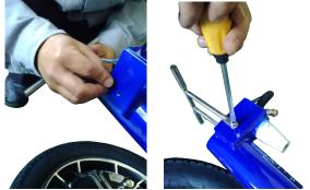
Open the spring with the screwdriver or other tool and then connect the spring to kickstand.
