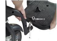
9. Prior to assembling or disassembling the Multi-Point AWD, place Multi-Point AWD on a flat surface, flip down the kickstand and ensure it is supporting the weight of the scooter.
