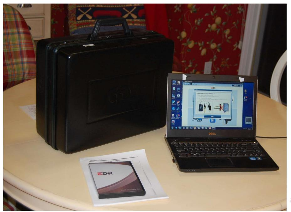
Kit consists of Vehicle Communication Interface (VCI), DLC Cable, Direct to Module Cables, Power Source.
