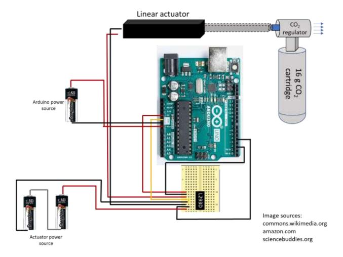
The actual robot also used an LCD screen and a potentiometer, but those are optional and are omitted for clarity.
