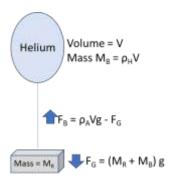
If the upward force  $F_B$  is nearly equal to the downward force of gravity  $F_G$ , we can create a microgravity environment.
