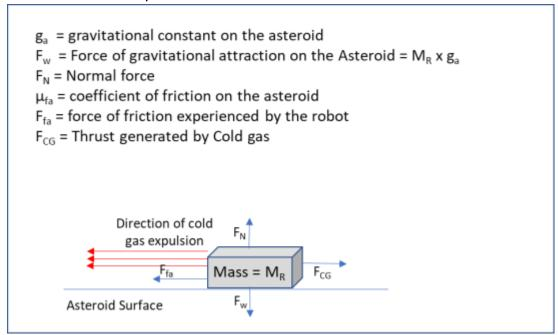
For the robot to be able to move, the thrust generated by the CG propulsion needs to be greater than the force of friction, i.e.  $F_{CG} > F_{fa}$ .
