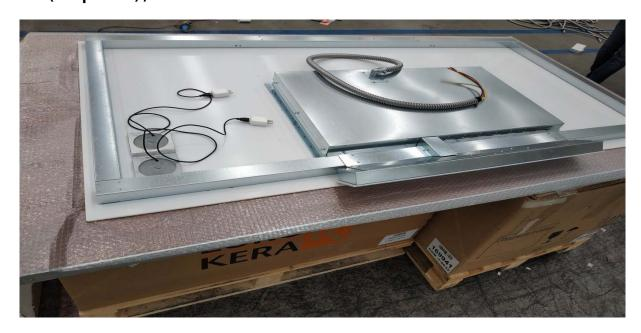
3. Unscrew the two screws and remove the cover (see picture)
