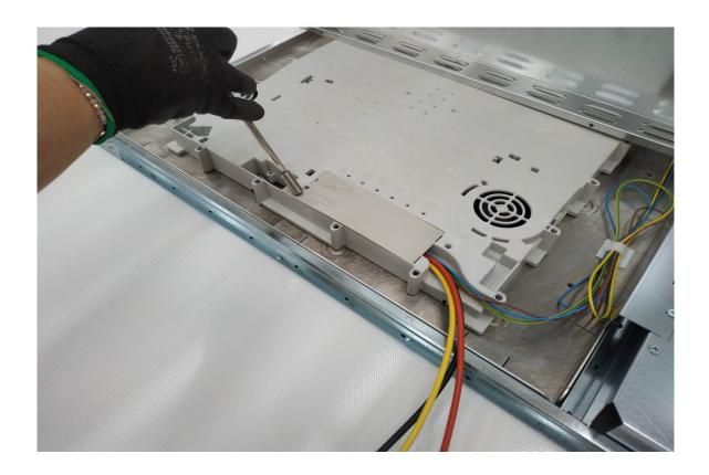
6.2 Disconnect the connections below (6 hexagonal and 1 Phillips screws) (see picture)
