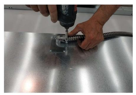
5. Unscrew the 12 perimetral screws of induction cover and remove it (see pictures)
