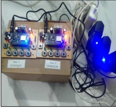
Figure 2. Experimental Prototype of the Multi-Zone IoT-Based Emergency Alert System Consisting of Two Monitoring Zones (Zone-1 and Zone-2) Using ESP8266 NodeMCU Controllers.
