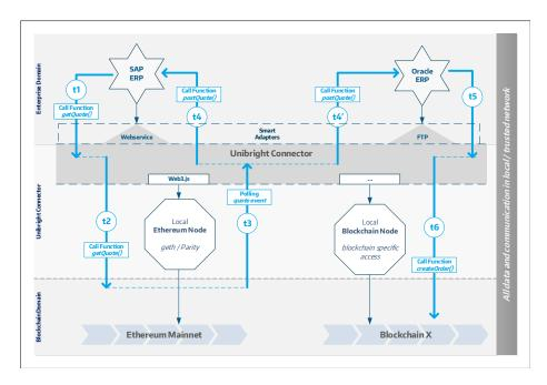
Figure 9: The Unibright Connector Architecture
