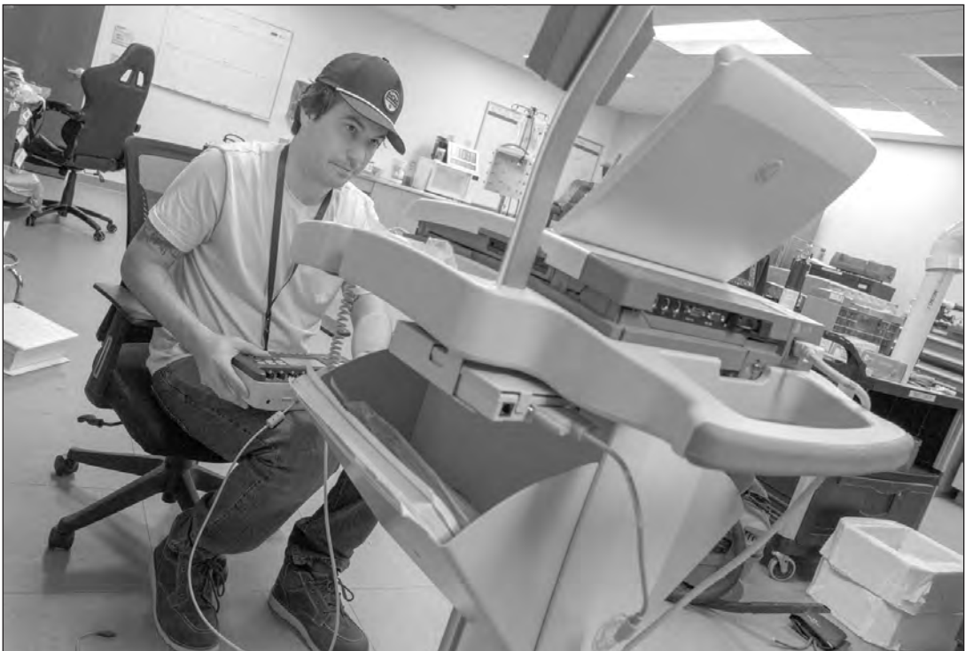
Stephen Danko, 78th Medical Group Healthcare Operations Squadron Biomedical Equipment Technician medical equipment repair technician, runs diagnostic testing on an electrocardiogram machine, or EKG, at Robins Air Force Base July 31. After testing, a defective internal wire was replaced, restoring the EKG machine to full operational capacity. (U.S. Air Force photo by Jerry Foltz)
