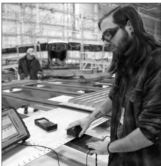
Dakota Holt, 558th Aircraft Maintenance Squadron nondestructive inspector, performs an eddy current array scan on a horizontal box beam panel for a C-5 aircraft horizontal stabilizer at Robins Air Force Base Dec. 10, 2025. The eddy current radius scan array checked for cracks and allowed NDI technicians to test the structural integrity of the aircraft skin. (U.S. Air Force photo by Joseph Mather)
