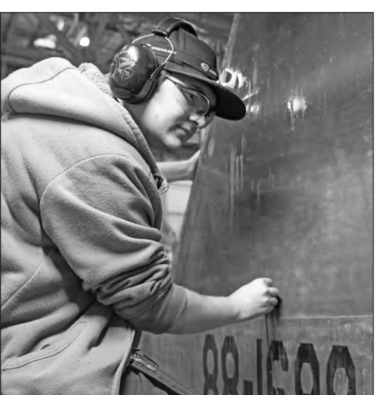
Ben Wheeler, 558th Aircraft Maintenance Squadron nondestructive inspector, performs an ultrasonic straight beam inspection delamination test to the outboard side of an F-15 aircraft stabilizer at Robins Air Force Base, Georgia, Dec. 10, 2025. NDI inspectors at Robins AFB tested the F-15 to assure the integrity of the aircraft as part of its programmed/scheduled depot maintenance. (U.S. Air Force photo by Joseph Mather)
