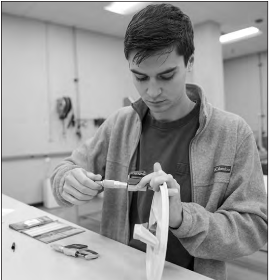
Michael Sottile, 802nd Maintenance Support Squadron Physical Science Laboratory mechanical engineer, uses a micrometer to check the thickness of a first article aircraft part at Robins Air Force Base March 25. The dimensional analysis was used to determine if the first article aircraft part matched the engineering drawings. (U.S. Air Force photo by Joseph Mather)
