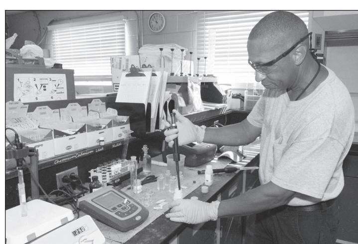
George Rackard, 78th Civil Engineer Squadron wastewater treatment plant operator, places a water sample into a cuvette to test for heavy metals in the wastewater at Robins Air Force Base Aug. 23. Eleven separate water sample tests were completed to determine treatment options to remove heavy metal from wastewater. (U.S. Air Force photo by Joseph Mather)
