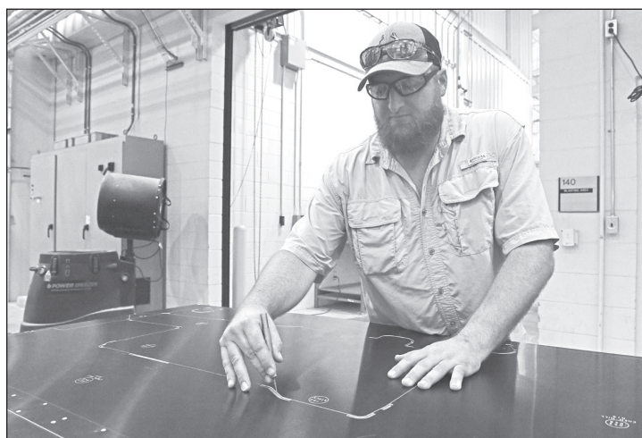
Daniel Honrath, 571st Commodities Maintenance Squadron metalizing equipment operator, uses an H-53 helicopter etching guide to cut the outline of various areas to be chemically milled on a piece of sheet metal at Robins Air Force Base June 21. The guide has specific measurements and milling instructions for the chemical milling process. (U.S. Air Force photo by Joseph Mather)
