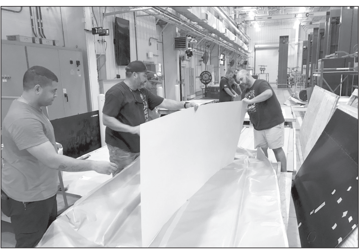
A team of maintenance workers with the 571st Commodities Maintenance Squadron Advanced Metal Finishing Facility, inspect a piece of sheet metal for defects at Robins Air Force Base Aug. 20. The United States Navy Fleet Readiness Center East requested the WR-ALC perform a one-time only chemical milling and anodizing process for 15 Navy H-53 helicopter skins. (U.S. Air Force photo by Danny Walters)
