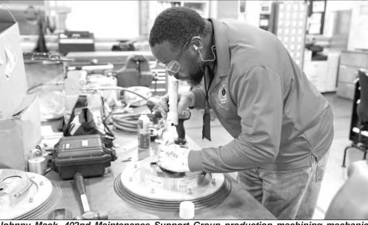
Johnny Mack, 402nd Maintenance Support Group production machining mechanic, makes repairs to a wing grip suction anchor for a C-17 aircraft at Robins Air Force Base May 21. The wing grips received annual preventive maintance to ensure the fall mitigation system is ready to be used to support the sustainment mission. (U.S. Air Force photo by Joseph Mather)
