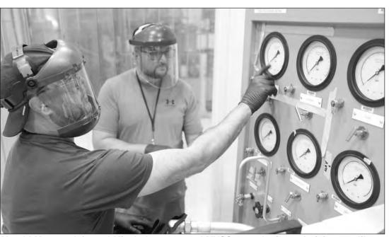
Harold Morrow, left, and Micah Jones, 802nd MXSS metrologist technicians, calibrate a Dowty Propellor pitch control test rig for the C-130J aircraft at Robins Air Force Base May 21. The metrology lab technicians performed on-site calibration of test measurement diagnostic equipment to ensure the overhaul and repair systems maintain sustainment standards. (U.S. Air Force photo by Joseph Mather)
