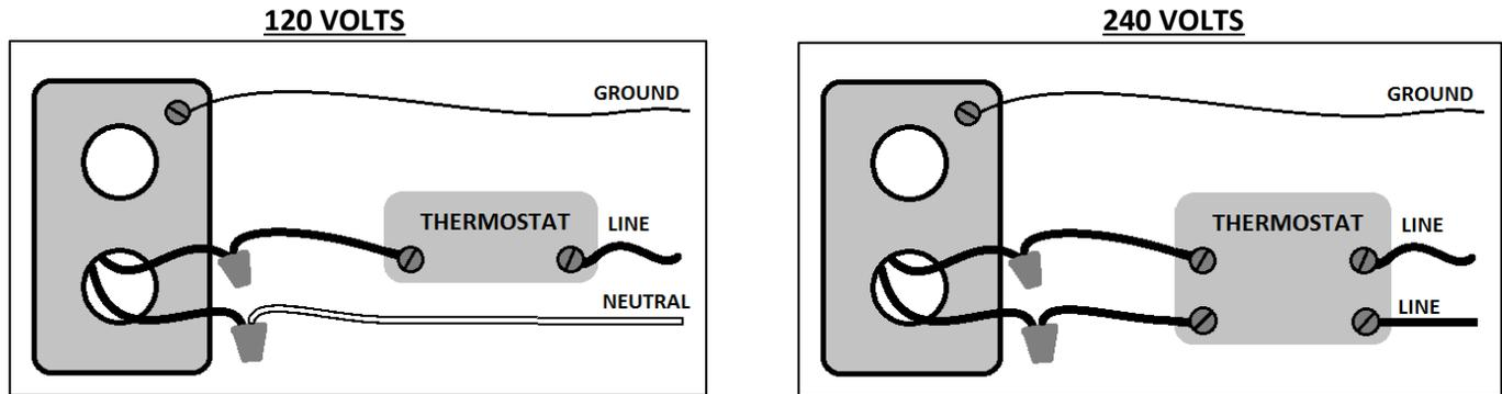
Figure 3 – Thermostat wiring connections for panels
