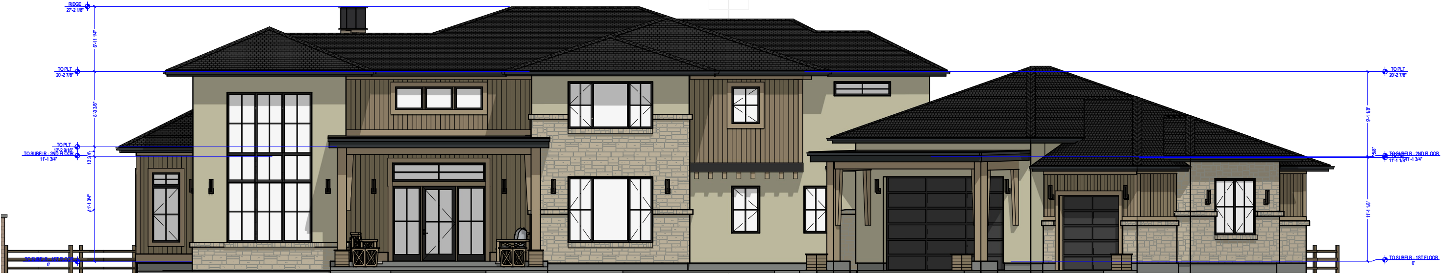
E1 EXTERIOR ELEVATION FRONT 10 1 IN = 10 FT
