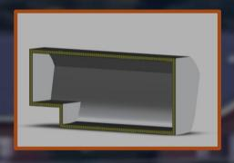
To meet the demands of ICARUS' performance, we are developing a Selective Laser Sintered Nylon 12 fuel tank. It will also serve as a major structural component. We will outfit it with optimized baffles, a robust level sensing system, and a hopper tank to provide consistent delivery in adverse conditions.
