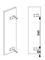
**Step: 5**Fix Shutter into frame with screw and tighten.
