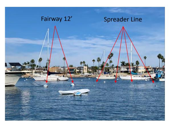
Closer view of fairway shows approximately 12 feet space to navigate through. Spreader line is longer than the mooring creating a safety hazard.
