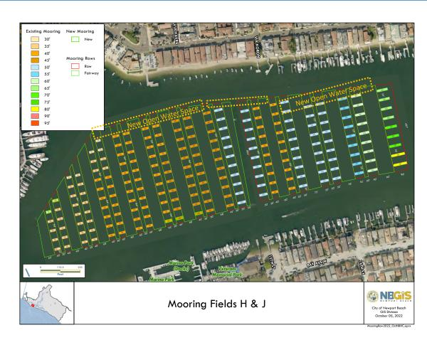
New configuration provides improved navigation and utilization of space. Only 11 boats per row vs 15. Every row is in substantial compliance with Harbor Design Standards 15-66
