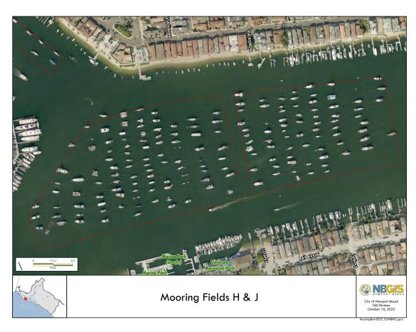
This is a poor utilization of space. Up to 15 boats in a row. Every row provides less than adequate spacing and is not compliant with Harbor Design Standards.
