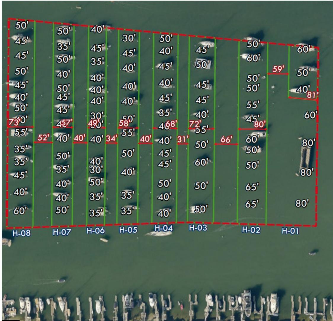
***Every row provides less than adequate spacing and is not compliant with Harbor Design Standards.***
