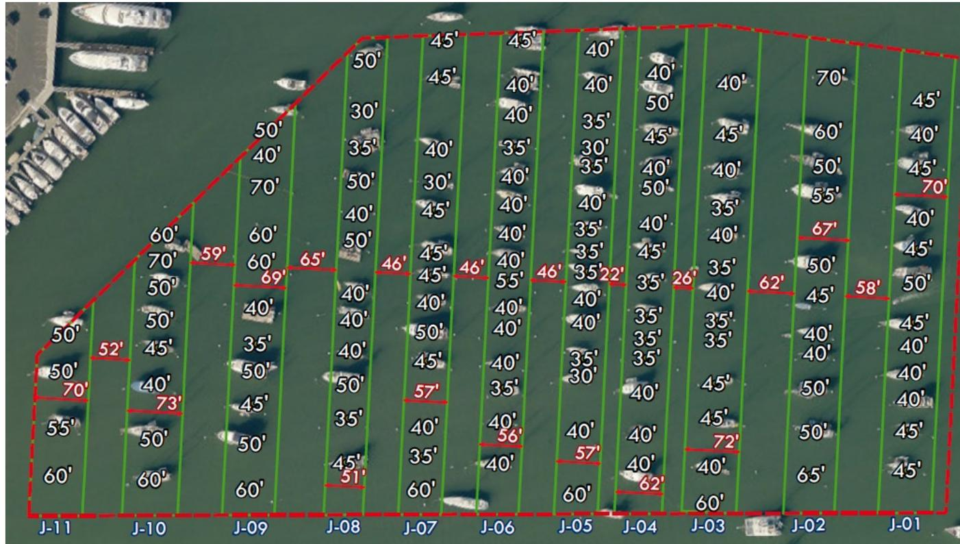
**Every row provides less than adequate spacing and is not compliant with Harbor Design Standards.**
