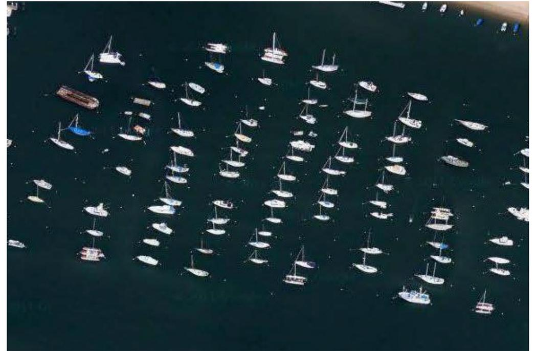
The typical 2-point mooring field above maintains consistent boat lengths in each row and clearly defined fairways for navigation. Newport Harbor mooring fields do not maintain consistency of boat lengths in rows or widths in fairways.
